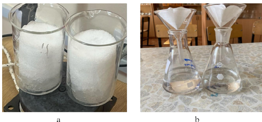
Figure 1 – a) Snowmelt process; b) Filtering process
