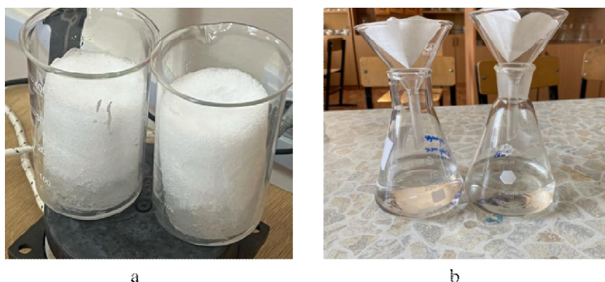
Figure 1 – a) Snowmelt process; b) Filtering process
